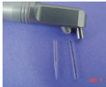
Figure 18. Laser delivery handpiece and sapphire tips
