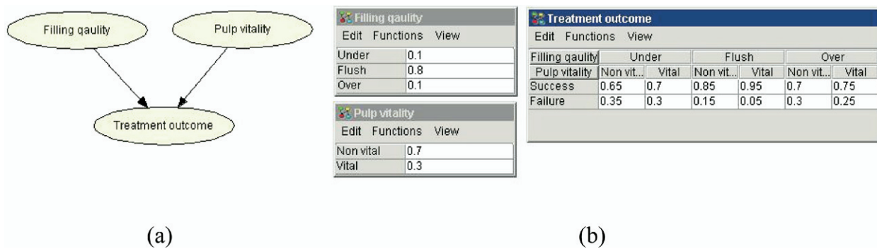
Fig. 2. (A) A simple Bayesian network. Each arc indicates a causal relationship. (B) Conditional probability table of treatment outcome. Because the node treatment outcome has 2 parents—pulp vitality and quality of root canal filling, this table contains probabilities of treatment outcome values, given the condition of pulp vitality and quality of root canal filling.
