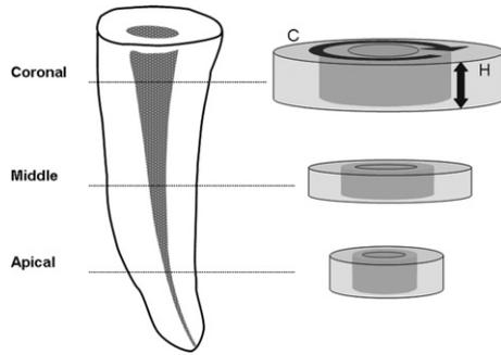
**Figure 1.** The roots were sectioned and ground to 0.7-mm-thick slices located at 3 different levels (coronal, middle, apical) inside the root. Each slice was placed in an apical-coronal orientation under the testing device to avoid the effect of variation in specimen conicity on the resistance to dislodgment. The push-out bond strength of each section was calculated as the force at failure divided by the bonded cross-sectional surface area (circumference [C] multiplied by height [H]).
