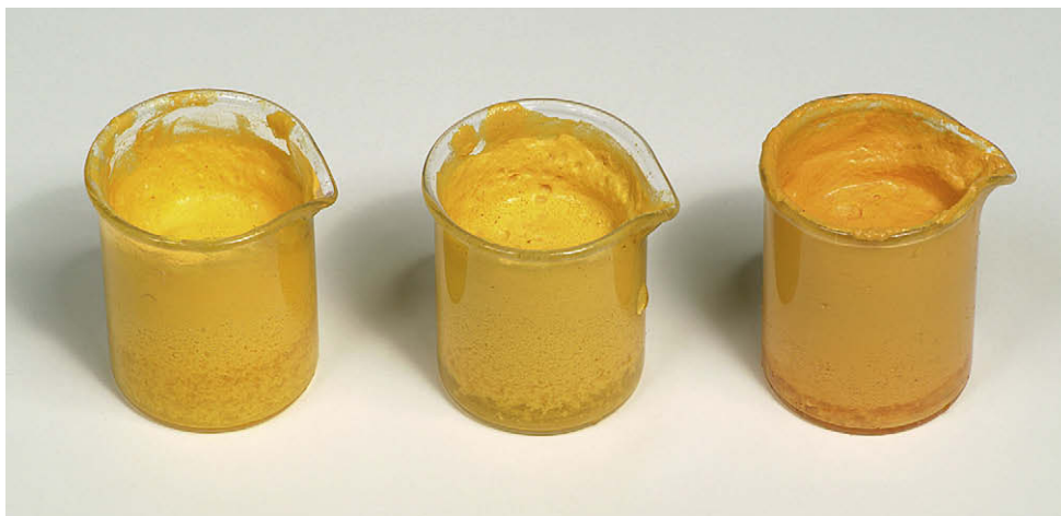
Figure 1. Tubes with aniline, PCA, and the NaOCl/CHX precipitate turned yellow, indicating that the amine was present.
