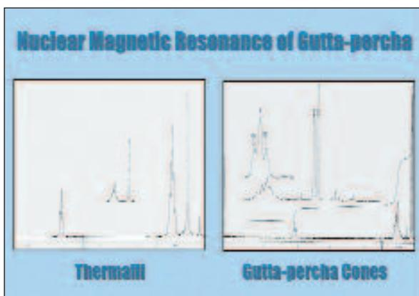
**Figure 9:** Infrared spectro-photometry of two types of gutta percha: conventional Thermafil and cones. The position and the extension of the peaks indicate the presence of alpha and beta phases and amorphous for the two types of gutta percha
