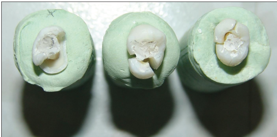
Figure 2. Occlusal view of three specimens following the fracture resistance test.
