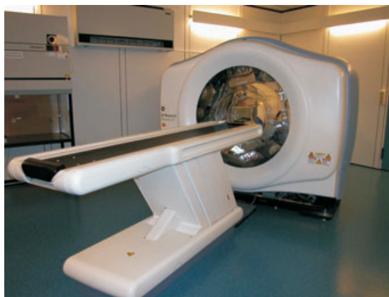
Figure 1 Prototype of the flat panel volume detector computer tomograph system, University of Göttingen, Germany.
