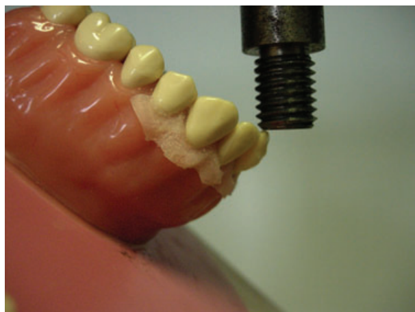
Fig. 4. Oblique 45° force and linear increasing intensity ranging from 0 to 30 N.
