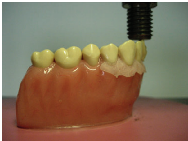
Fig. 3. Axial load and linear increasing intensity ranging from 0 to 50 N.
