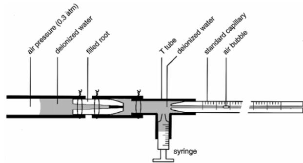
Fig. 2. Fluid transport device for leakage determination.
