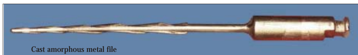
Fig. 40 Liquidmetal cast file (the handle and shaft are cast as one piece). Casting allows the blades to be designed to spiral only 180 degrees around the shaft in order to reduce canal wall engagement. It also allows each blade to have a different helix angle to avoid screwing-in forces. Continuous advancements in casting techniques can make it a viable manufacturing process in the near future.
