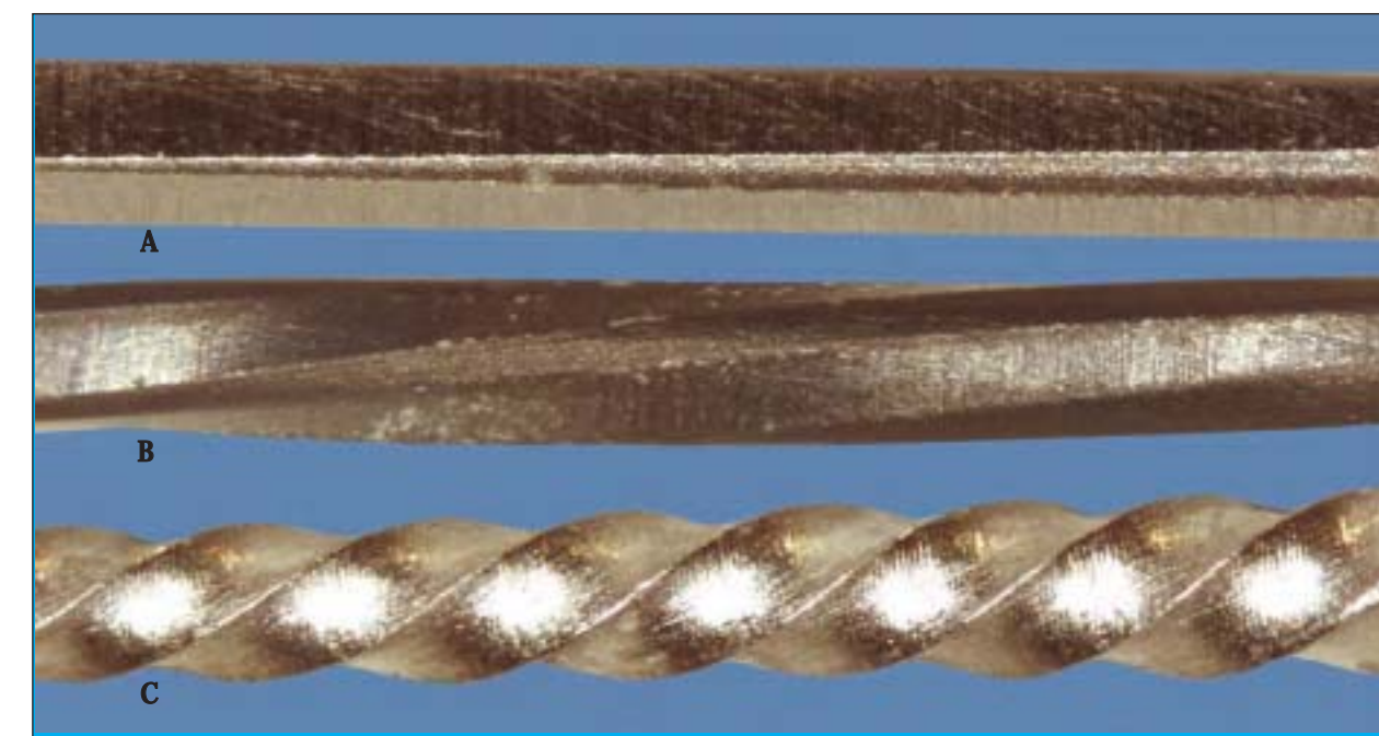
Fig. 2 A. A tapered pyramidal wire is used as a blank for forming a file. B. Each end of the blank is stabilized and one end is rotated to twist a spiraled shape on the file's working surface. C. Multiple rotations result in the familiar spiraled shape of the endodontic file.
