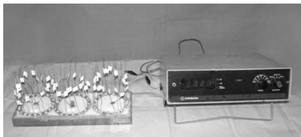
**Figure 1** Apical leakage test system for the electrochemical method.
