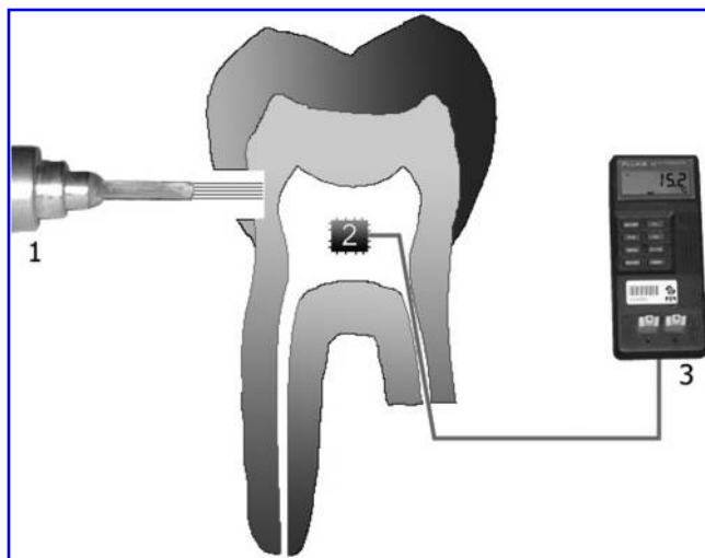
FIG. 1. Experimental model showing the position of the thermocouple inside the pulp chamber. 1 = laser; 2 = thermocouple in pulp chamber; 3 = thermometer.
