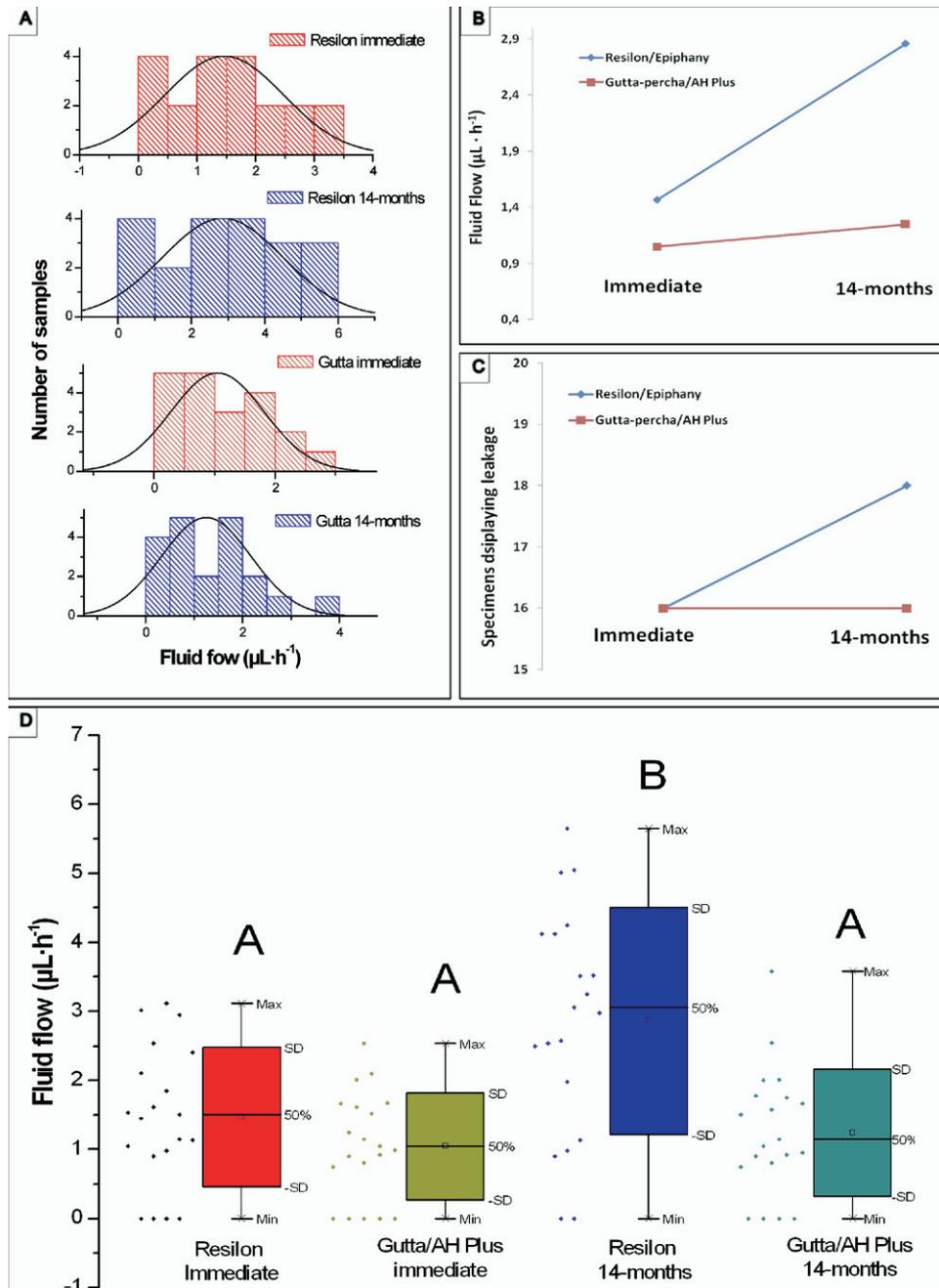
**Figure 2.** (A) Histograms for each group to show the intrinsic dispersion of the data at the initial measurement and 14 months later. (B) Fluid flow measures and (C) the number of specimens that show detectable leakage. (D) Box plots of the fluid flow data at the initial measurement and 14 months later; letters indicate significant differences between groups;  $P < .05$ .
