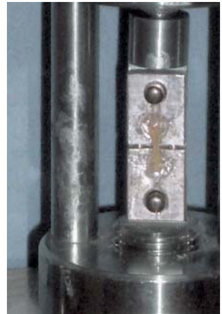
Fig 4 Mounting of a study sample on the universal testing machine.
