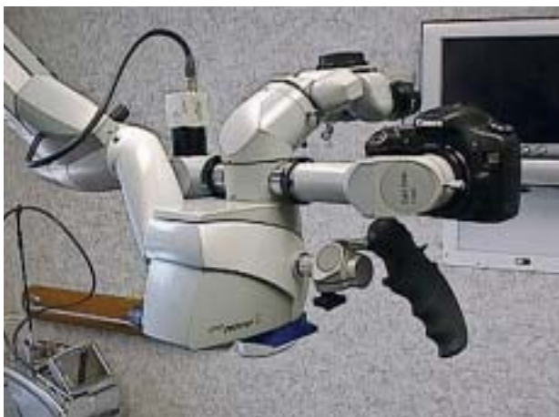
Fig 19 Canon SLR camera on the left side of a Zeiss ProErgo microscope and a medical-grade cube camera on the right side. (Photograph courtesy of Dr Wade Karhan, Rittman, Ohio.)
