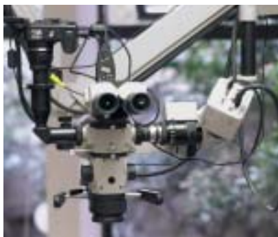
Fig 18 Nikon 5000 point-and-shoot camera on the left side of a Global G6 microscope.
