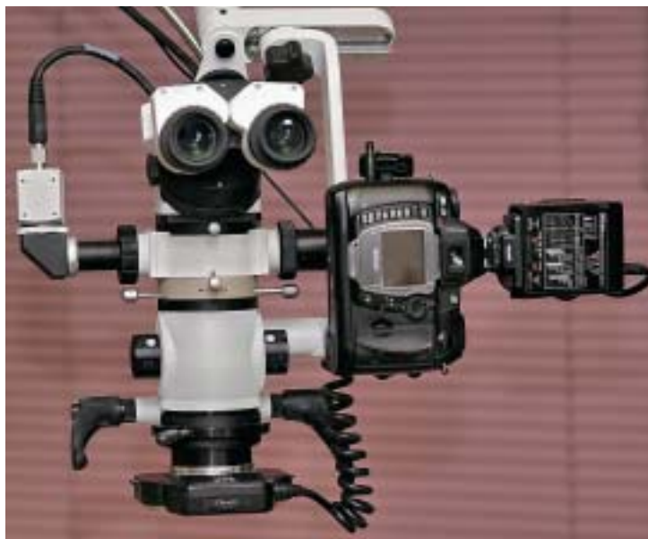
Fig 3 Microscope with Nikon Digital SLR camera on the right side, a Nikon SB-29 ring flash mounted at the bottom, and a Sony three-chip digital medical-grade cube camera on the left side.
