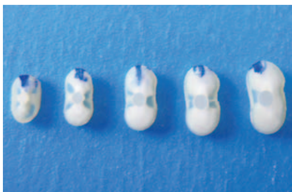
Fig 1 1-mm-thick root slices containing the bonded fiber post prior to push-out testing.
