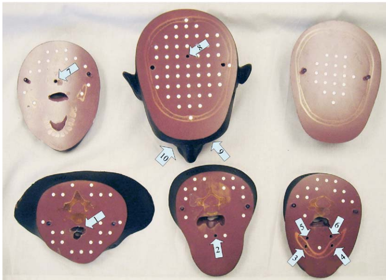
Fig. 3. A total of 10 thermoluminescent dosimeters (TLD) were used for this project. Besides the 8 shown in this image, there were 2 additional TLDs taped to the phantom's eyes.
