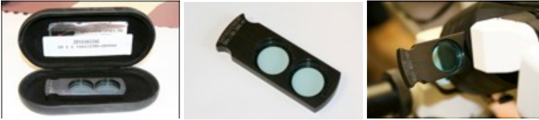
Fig 13a ErYAG microscope laser filter Fig. 13b Light blue ErYAG filter. Fig 13c Filter in scope.
