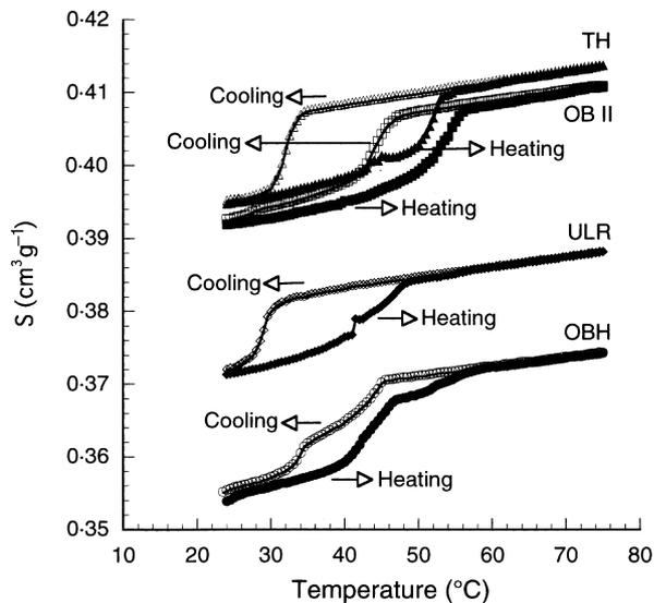
**Fig. 3.** Variation of specific volume (*s*) with temperature of four materials (heating and cooling rate: 0.5°C/min).
