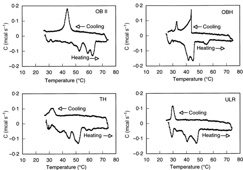
**Fig. 4.** Variation of Quantity of heat (*c*) with temperature of four materials (heating and cooling rate: 0.5°C/min).
