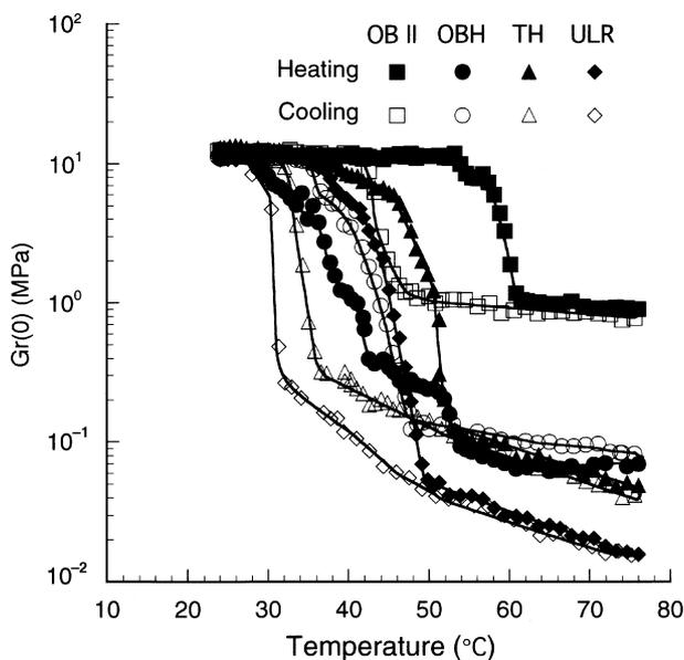
Fig. 2. Variation of Gr(0) with temperature of four materials (heating and cooling rate:0.5°C/min).
