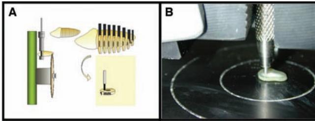
**Figure 1.** (A) Dentin disk preparation using an Isomet saw, (illustration courtesy of Teixeira FB, Levin LG, and Trope M). (B) A 1.2 mm punch being lowered onto 1.0 mm dentin disk in SATEC universal testing machine.
