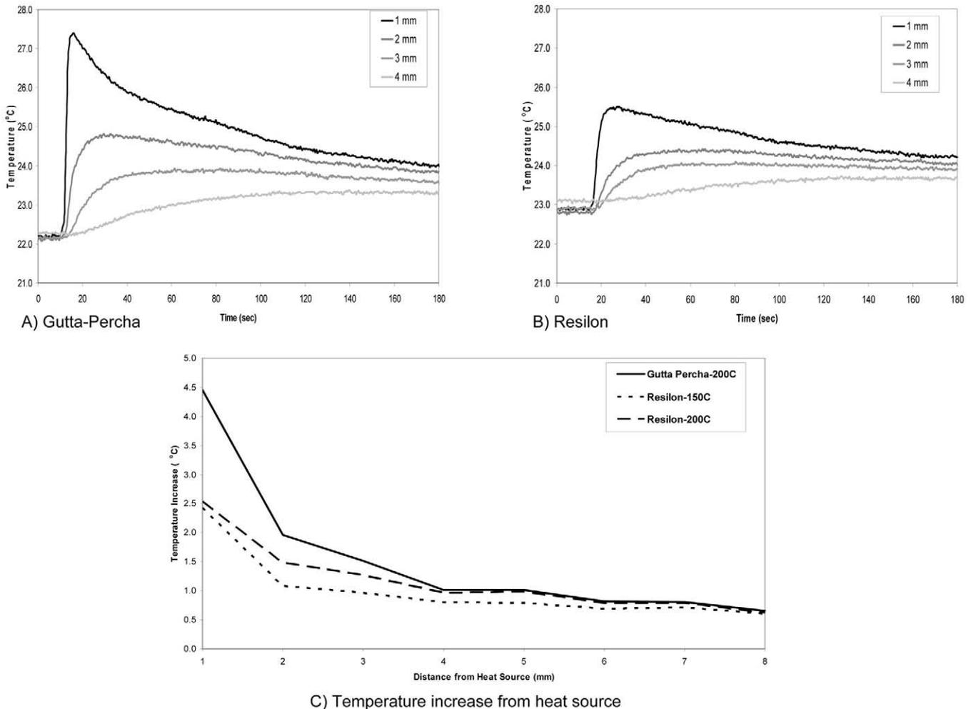
Figure 3. (A) Heat transfer test for gutta-percha. (B) Heat transfer test for Resilon. (C) Temperature increase from heat source, gutta-percha, and Resilon.
