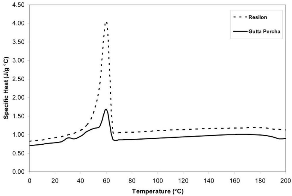
Figure 2. Specific heat capacity for gutta-percha and Resilon.
