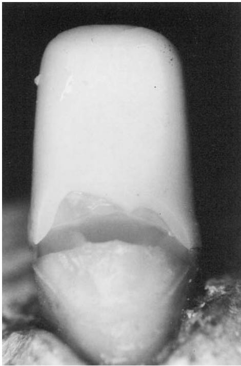
FIG 6. Failure of a specimen in the Zwick testing machine (group C).
