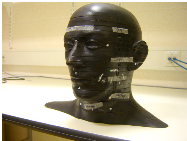
Fig. 3. Anthropomorphic Rando ® Alderson phantom, used for measurements on the CBCT devices. Only the 20 slices which were used for TLD placement are shown.
