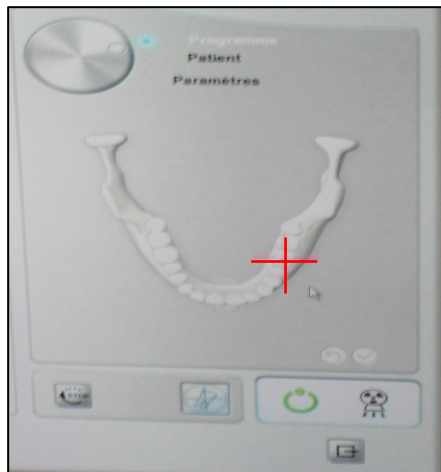
Figure 2: Centring of the zone to be explored on the control station panel (the axis of rotation is represented by the red cross).
