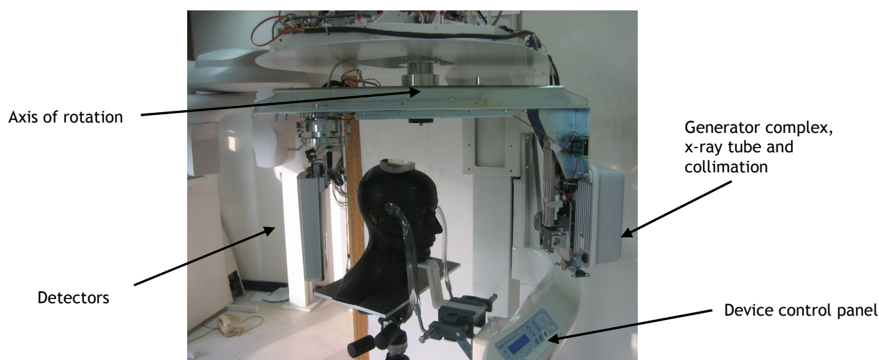
Photo 1: Main components of the Kodak 9000 3D device (housing removed)
