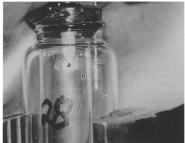
Fig 2. A drop of irrigant (a) suspended from the apical end of the root in the assembled apparatus before falling into the collection vial (b). Flask (c).
